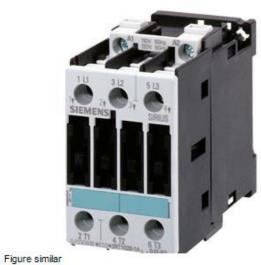
CONTACTOR, AC-3 11 KW/400 V, DC 24 V, 3-POLE, 2 NO + 2 NC, SIZE S0, SCREW CONNECTION
